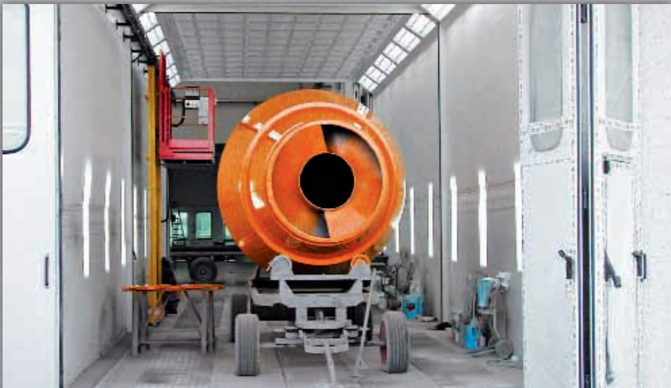
VISTA INTERNA GL5 CON BASAMENTO IN OPERA MURARIA A 3 FILE DI GRIGLIE, PREDISPOSTO PER MEZZI PESANTI INSIDE VIEW OF GL5 WITH MASONRY WORKS WITH THREE ROWS OF GRIDS CONCEIVED FOR HEAVY VEHICLES
