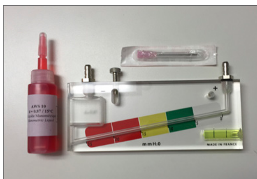
OPTC061 KIMO pressure gauge for internal pressure monitoring
