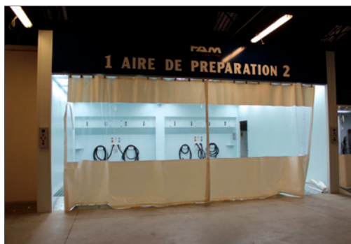
OPTZP014 Manual curtain (horizontal opening) h. max. 3,5 m /m 2
