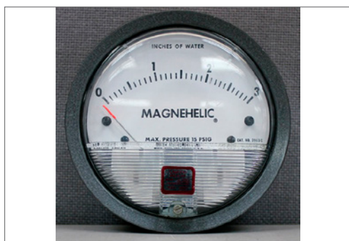
OPTC060 Magnehelic pressure gauge for internal pressure monitoring
