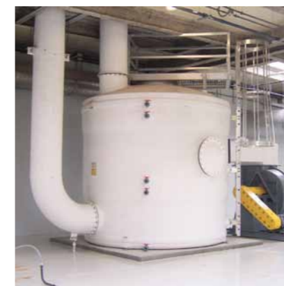
Symbolfoto: Purafil® ESD Vessel Scrubber
